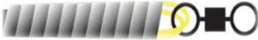
Pulling eye for fiber optic cable attached by strength members
